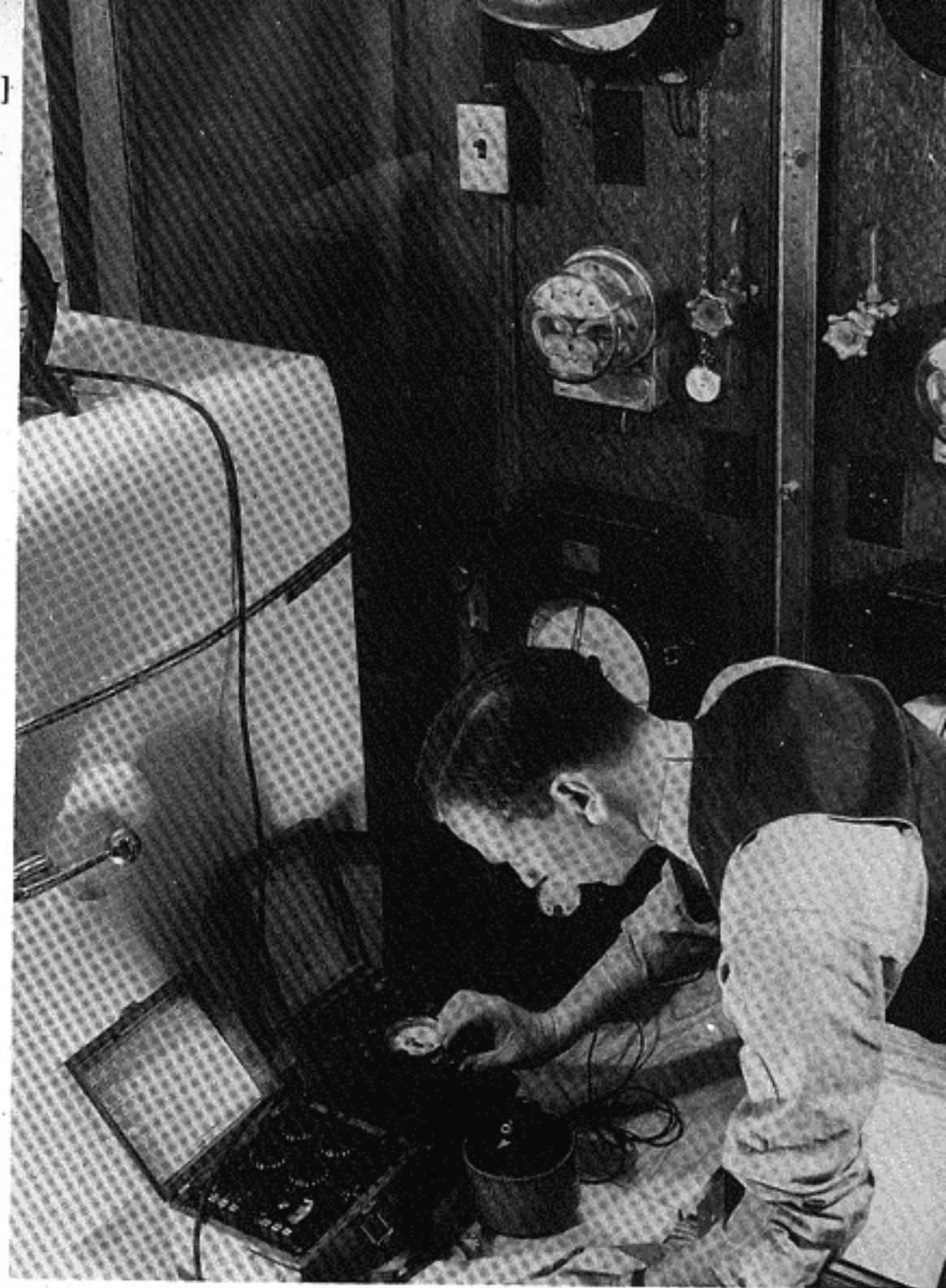
A research engineer at the Sunbeam Electric Manufacturing Co. tests a Coldspot refrigerator, with the calorimeters recording the performance of the unit under various loads.
