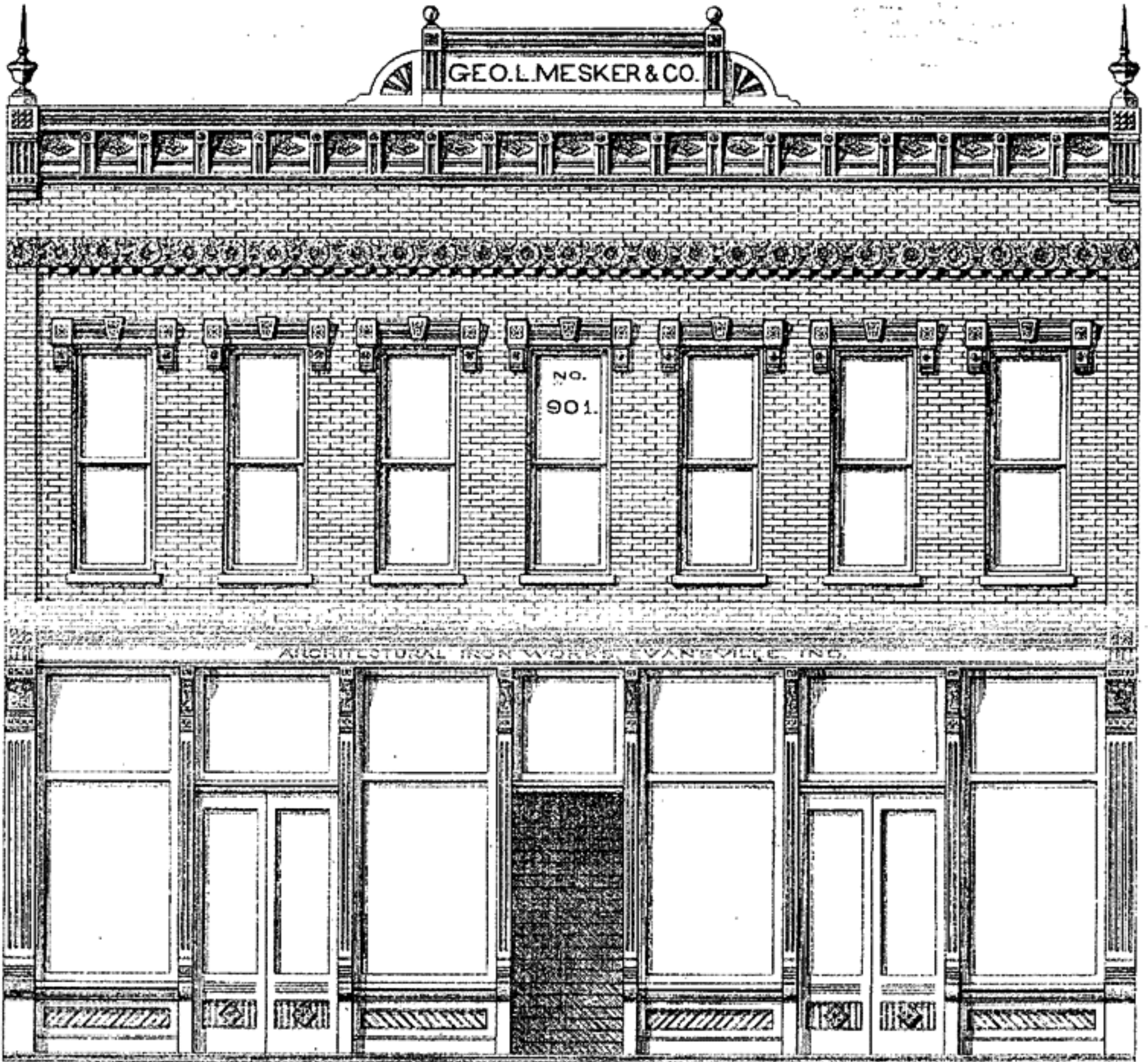
No. 901. Galvanized iron lintel cornice, main cornice, pediment, scrolls, urns and window caps, for 40 ft. front. $116.15. Belt course extra.
